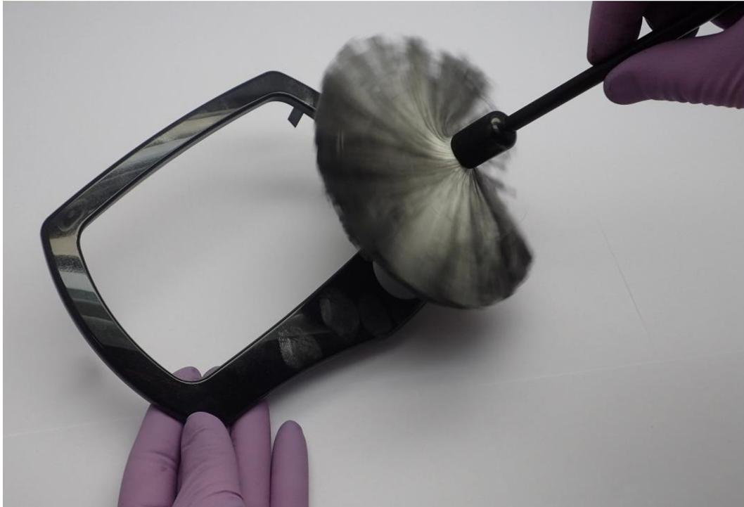
Figure 2: Wetting of the part with *Contamination Spy* powder by a rotating movement of the zephyr brush
