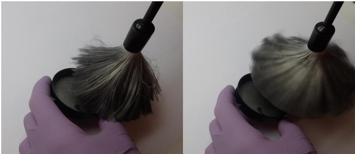
Figure 1: Wetting of the zephyr brush with the *Contamination Spy* powder, which adheres on the cap of the product vessel
