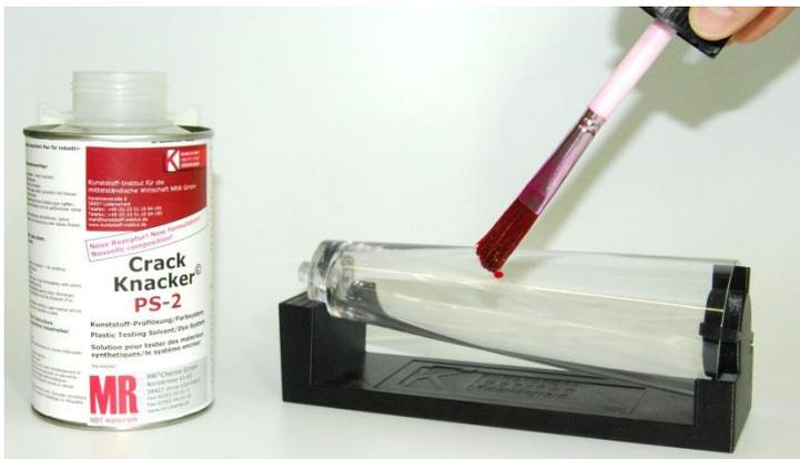
Figure 1: Application of Crack Knacker<sup>®</sup> using brush (source: Kunststoff-Institut Luedenscheid)
