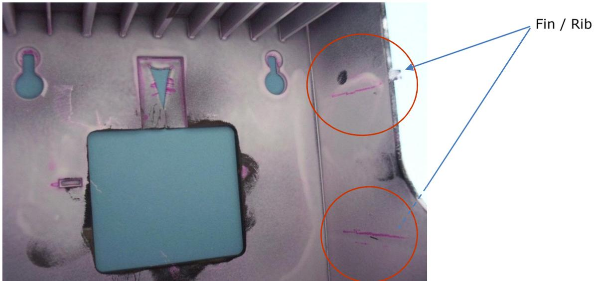
Figure 2: „CD-Stack-box“, residual stresses in the area of fins or ribs (source: Kunststoff-Institut Luedenschied)
