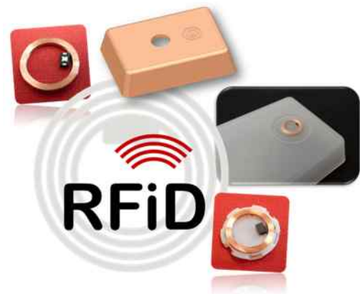
RFID tag, 3D model of demonstrator part, molded part with integrated RFID tag, RFID tag in carrier module (left to right)
